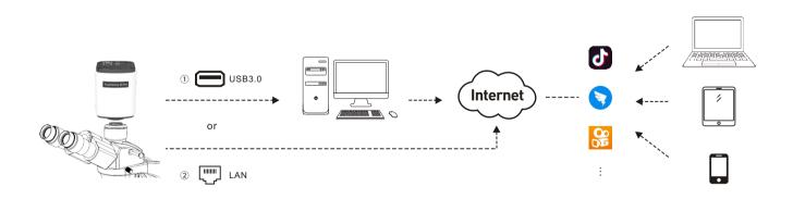
Remark: ① USB 3.0: can perform voice interaction under the help of computer audio function. ② LAN: No simultaneous voice interaction supported since no audio interface on camera.
