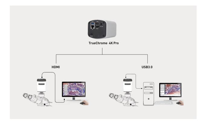
TrueChrome 4K Pro is one microscope camera mixing HDMI shortcut operation and USB 3.0 professional software analysis.
